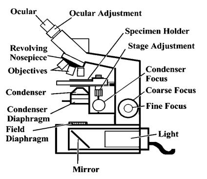
After putting the slide on the stage of the microscope, the light is turned on and the specimen must be observed and put into focus with the objective that has the smaller magnification. This is done by using first the coarse focus knob and only when the image is roughly focused the fine focus knob. Once the specimen is in focus we can change objective to one with higher magnification. Once the next objective is in place we will need to use only the fine focus knob to visualize the specimen.
